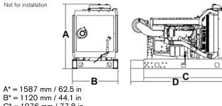
$C^* = 1976 \text{ mm} / 77.8 \text{ in}$ D = 2296 mm / 90.5 in (During transport)
